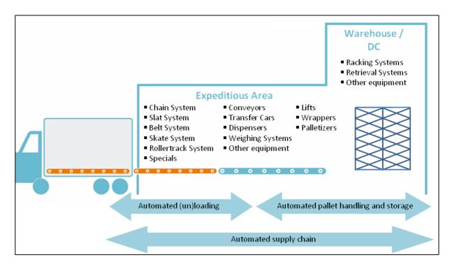
The ATLS and the internal conveying systems can be connected and enable a fully automated supply chain.
