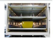
Baur Versand is part of the Otto Group and is a major internet retailer and mail-order company in Germany. Ancra Systems have installed an automatic trailer loading/unloading system in three swap bodies. The swap bodies are shuttled ( $\pm$  2 km) between the computer controlled central warehouse and the distribution centre where orders are picked.
