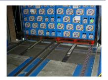
Bavaria NV is one of the oldest and biggest breweries of The Netherlands, serving an international sales area. At the headquarters in Lieshout, Ancra Systems delivered and installed a chain conveyor dock system, allowing fluent and efficient shuttle transport between the beer production facility and the newly built distribution centre.
