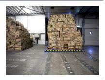
J. van de Put Fresh Cargo Handling is a company located near Schiphol Airport for fast handling of fresh products such as flowers, plants, fruits and vegetables. Ancra Systems BV made it possible for Van de Put BV to deliver high quality products by installing pneumatic rollertracks for rapid air cargo handling.
